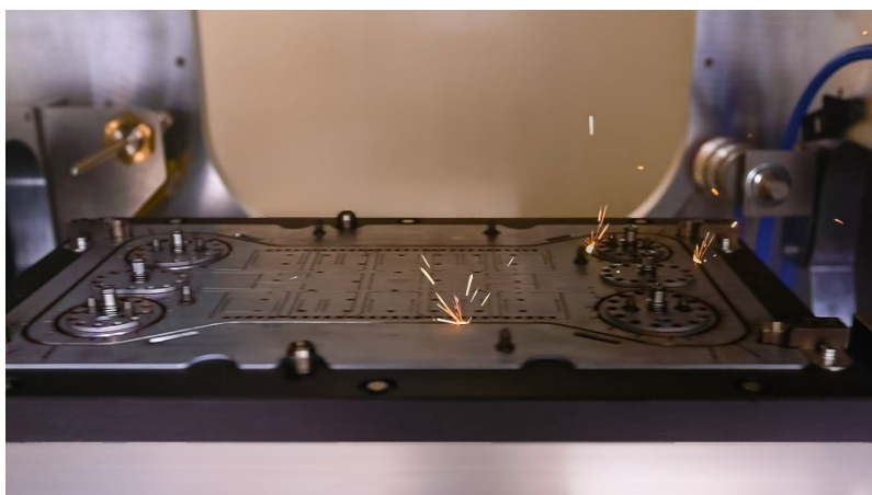
Multi-scanner (Galvo-Laser), on-the-fly welding
